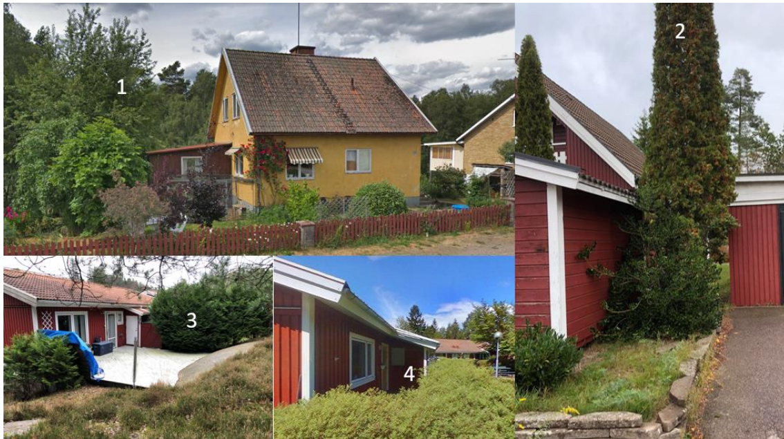
Figure 32. Some examples of vegetation fuels in gardens. (1) Plaster house with wooden extension on a garden with lots of deciduous and not very flammable ornamental plant. The forest behind is coniferous except for trees just adjacent to the garden. (2) Wooden single dwelling with nearby garage and storage outbuilding and two large Thuja Occidentalis next to the façade. (3) Cupressus leylandii growing up to wooden façade and deck at suburban townhouse. The vegetation around is dominated by Calluna . The photo is taken during autumn and residents confirm that the deck is filled with tables and chairs during summer season. (4) suburban townhouse surrounded by Dasiphora fruticosa , commonly called Tundra rose (Ölandstok – Swedish).
