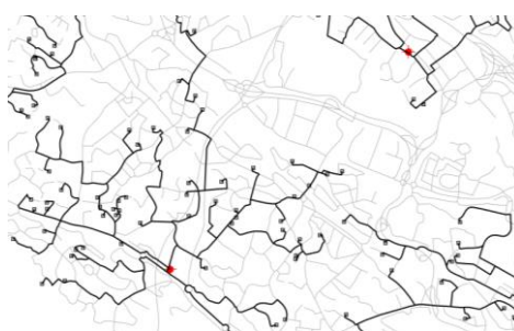
Figure 1. Excerpt from the road network analysis. Black squares represent sample buildings from the high-density population and the red circles fire stations.
